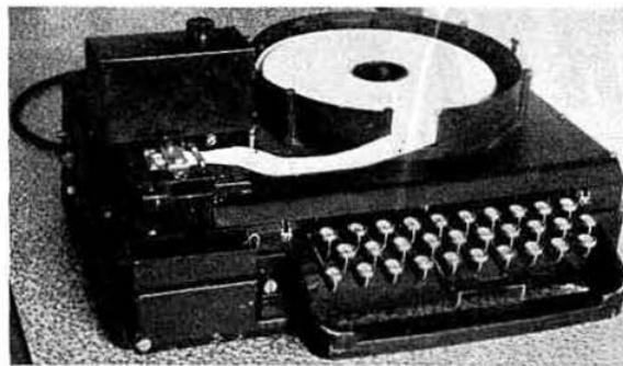
The Teleprinter Perforator No. 44 used by the GPO for many years. Machines of this type are frequently available on the surplus market.
